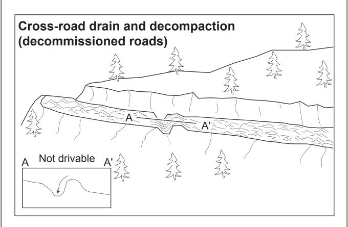
Cross road drain construction will ensure gullies, springs, road runoff and other concentrated flow will no longer collect over long lengths of road causing gully erosion and sediment delivery to streams. Cross road drains will be constructed at approximately 75 ft spacing intervals and these cross road drains will direct road surface runoff off the road onto stable hillslope locations.
