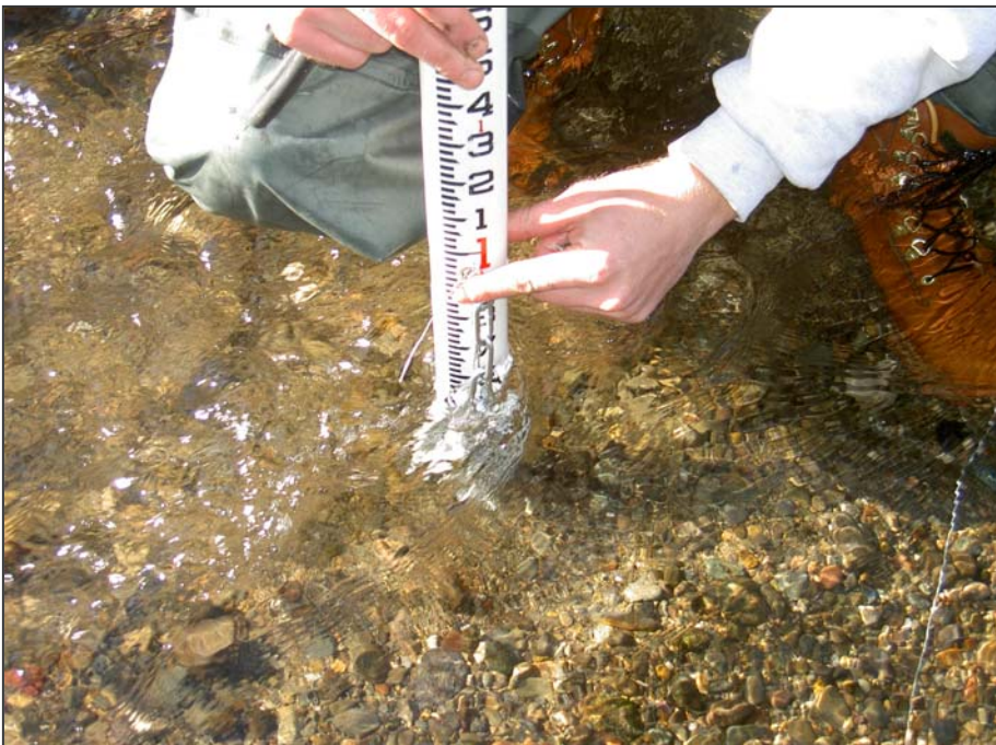
Measuring the scour chain's exposed length from the substrate with a stadia rod.
