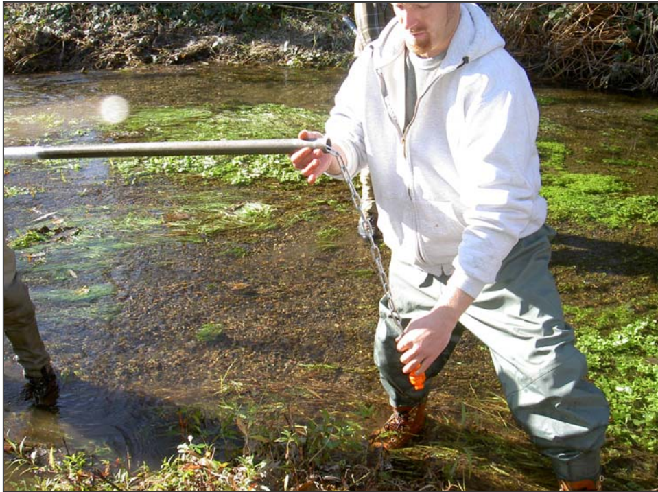
Scour chain being placed into the steel installation pipe
