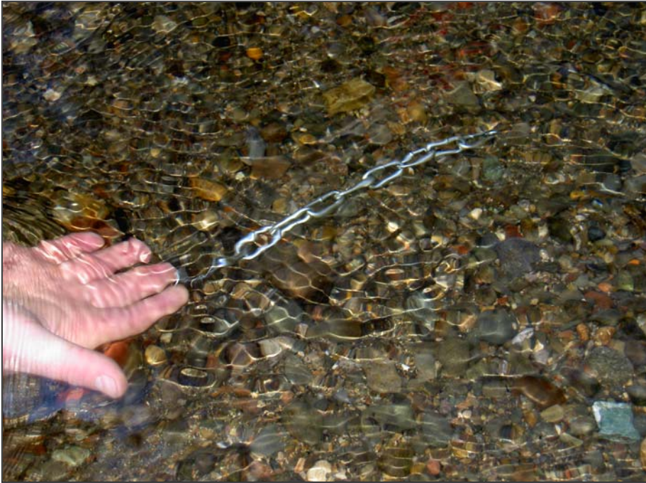
Installed scour chain after being driven into the streambed.
