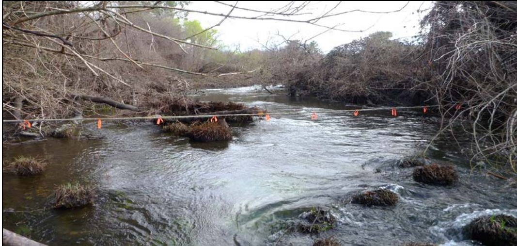
Figure 8. PIT tag antenna across the Napa River - destroyed during water year 2016-17.
