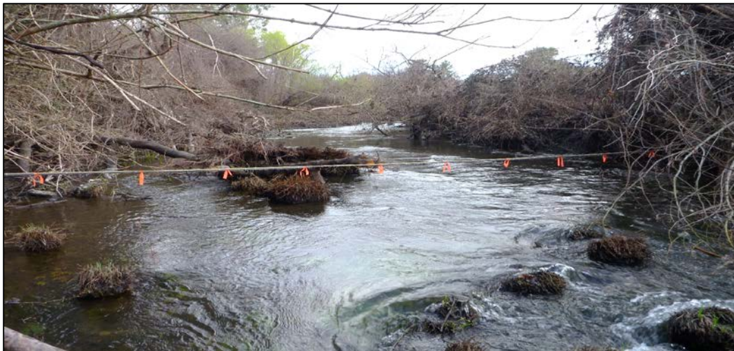
Figure 9. PIT tag antenna across the Napa River. Note, the lower portion of this “swim-through” loop runs along the bed of the river, and is not visible under the water.
