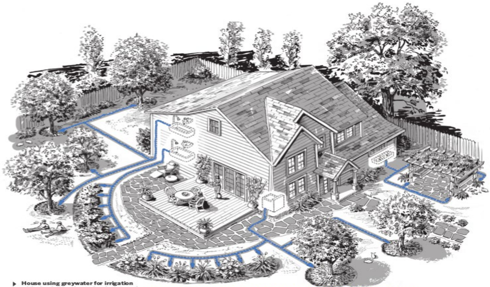
► House using greywater for irrigation with simple laundry-to-landscape and gravity-fed systems
